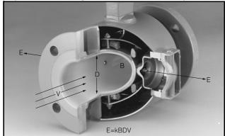
Magnetic field coils placed on opposite sides of the pipe generate a magnetic field. As the conductive process liquid moves through the field with average velocity V, electrodes sense the induced voltage. The width of the conductor is represented by the distance between electrodes. An insulating liner prevents the induced voltage signal from shorting to the pipe wall.
