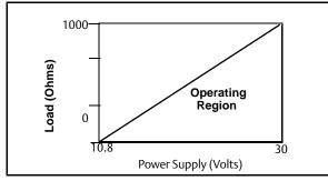
R\_max =52.08 (V\_{ps} - 10.8)V\_{ps} =Power Supply Voltage (Volts)R\_max =Maximum Loop Resistance (Ohms)
