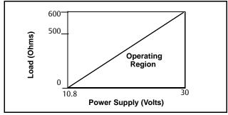
R<sub>max</sub> = 31.25 (V<sub>ps</sub> - 10.8) V<sub>ps</sub> = Power Supply Voltage (Volts) R<sub>max</sub> = Maximum Loop Resistance (Ohms)
