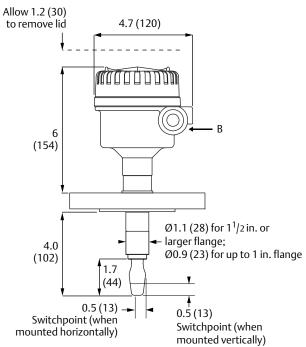
A. Cable entry M20 x 1.5 or  $^{1}$ /2-in. ANPT B. Cable entry M20 x 1.5 or  $^{3}$ /4-in. ANPT
