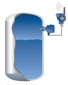
Wireless applications using a Rosemount 702 Discrete Transmitter
