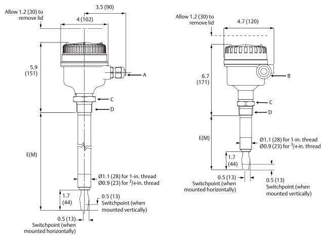
A. Cable entry M20 x 1.5 or  $^{1}/_{2}$ -in. ANPT B. Cable entry M20 x 1.5 or  $^{3}/_{4}$ -in. ANPT
