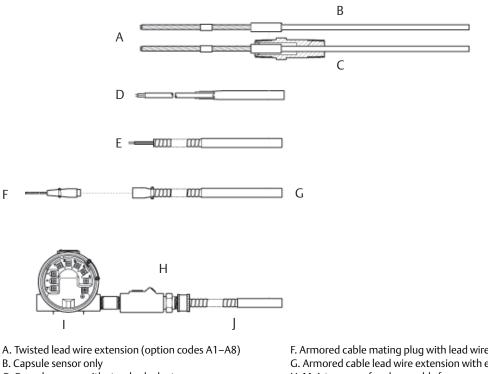
C. Capsule sensor with standard adapter D. Shielded cable lead wire extension (option codes B1-B8)
