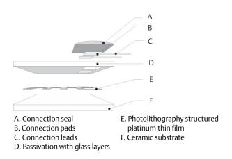
Design and construction of the Rosemount Series 68 Platinum Sensors provides the optimum combination of accuracy and durability available for temperature measurements. The construction of the sensor allows for direct immersion in non-corrosive fluids at reasonable static pressures. For corrosive environments or many industrial applications, these sensors are widely used with standard thermowell assemblies.
