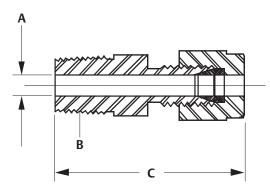
A. Fitting diameter B. Sensor process thread C. Length
