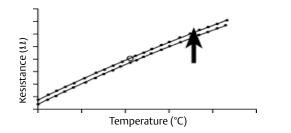
A one-point trim shifts the ideal curve up or down based on the single characterized point.
