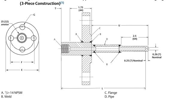
Figure 41. Flange Mounted Thermowells - Stepped, For Thermowells with Overall Length greater than 42-in.
