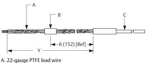
B. PTFE C. Sensor Dimensions are in inches (millimeters).
