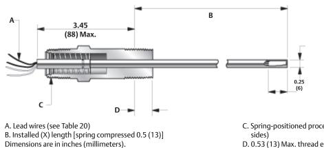
C. Spring-positioned process mounting connection (1/2-14 ANPT, both
