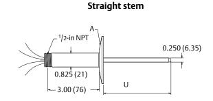
A. Tri clamp endcap B. Stem Dimensions are in inches (millimeters)
