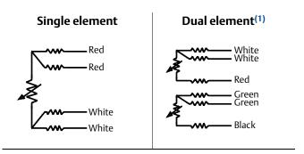
1. Dual element sensors are only available on Rosemount Series 68Q and 78 Sensors.
