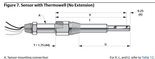
A. Sensor mounting connection Dimensions are in inches (millimeters).
