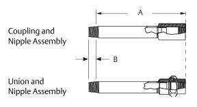
A. Length (E) (nominal) B. 0.53 (13) Max. thread engagement (<sup>1</sup>/2–14 ANPT Ref.) Dimensions are in inches (millimeters).
